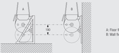
A: Floor fixing (optional) B: Wall fixing (standard)
