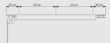
This motor is enormously strong and both fixing points and ceiling must be accordingly solid. Timber soffit at least 4cm thick over complete length of track is recommended.
